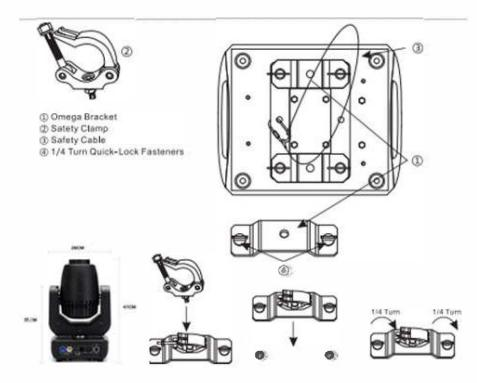
Regardless of the rigging option you choose for your LED moving head, always be sure to secure your fixture with a safety cable. The fixture providers a built-in rigging point for a safety cable on the hanging bracket as illustrated above. Be sure to only use the designated rigging point for the safety cable and never secure a safety cable to a carrying handle.
