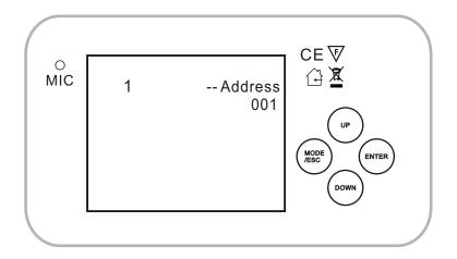
Press the <UP>or<DOWN>button repeated until you reach the desired menu function. Press the <ENTER>button to select the menu function currently displayed, or to enable menu option. To reture the previous option or menu without changing the value.Press the<MODE/ESC>button
