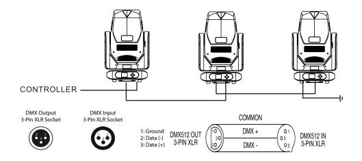
For installations where the DMX cable has to run a long distance or is in an electrically noisy enviromentsuch as in a disco, it is recommended to use a DMX terminator. This helps in preventing corruption of the digital control singal by electrical noisy. The DMX terminator is simply an XLR plug with a 120 resistor connected between pins 2and 3, which is then plugged into the output XLR Socket of the last fixture in the chain. Please see illustrations
