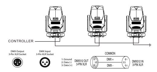
For installations where the DMX cable has to run a long distance or is in an electrically noisy environments as in a disco, it is recommended to use a DMX terminator. This helps in preventing corruption of the digital control singal by electrical noisy. The DMX terminator is simply an XLR plug with a 120 resistor connected between pins 2 and 3, which is then plugged into the output XLR Socket of the last fixture in the chain. Please see illustrations
